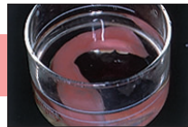
10) Immersion in RESIN HARDENER II solution (for more than 3minutes)
